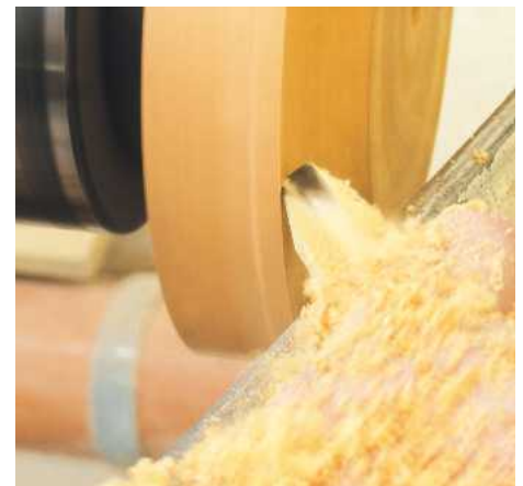
▲ Pic.9 Shape the base with a pull cut with the gouge, this being the quickest way to remove timber. If the flute of the tool is too shut you will blunt the tool quickly
